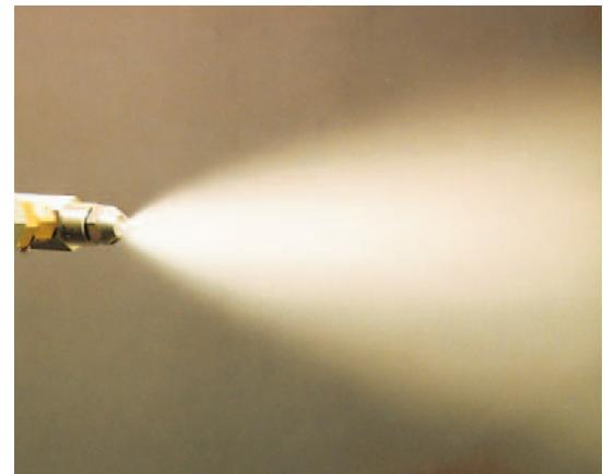
Ultrasonic atomizers can only be manufactured with high precision machining operations but offer the following remarkable advantages:
